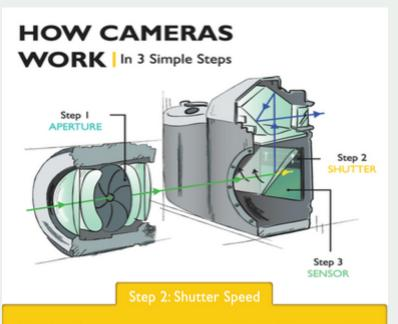
The mirror flips up and the shutter opens, recording the light present onto the sensor (or film). The speed at which this happens determines the exposure length as well as the amount of motion blur.
